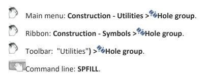
Universal command for drawing holes. With its help, you can draw a new hole with centerlines, or by specifying a group of holes to assign them general properties with filling of a sector.
