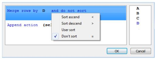
4. Click *OK* to check the result in the table editor. Cells having identical values in the D column will be merged.
