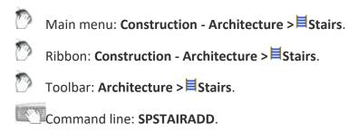
Stairs include linear and arc segments. For building arc section you need to select *Arc* in context menu.
